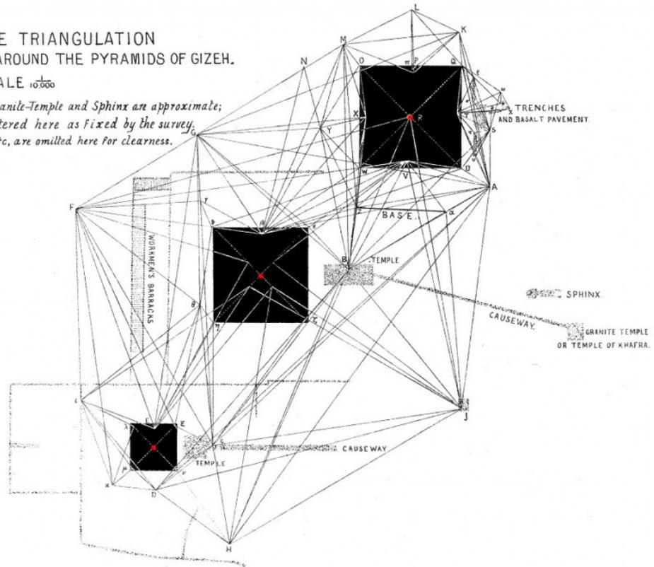
PLAN OF THE TRIANGULATION OF THE SURVEY OF 1881 AROUND THE PYRAMIDS OF GIZEH.
